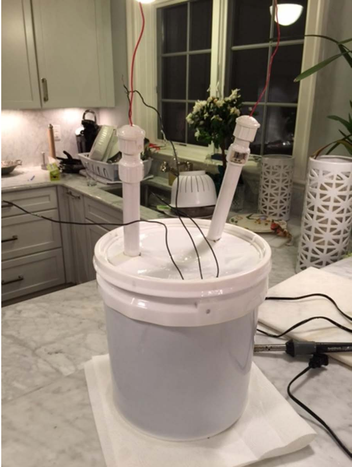
X-Ray Transformer with Rectifier Under Oil
