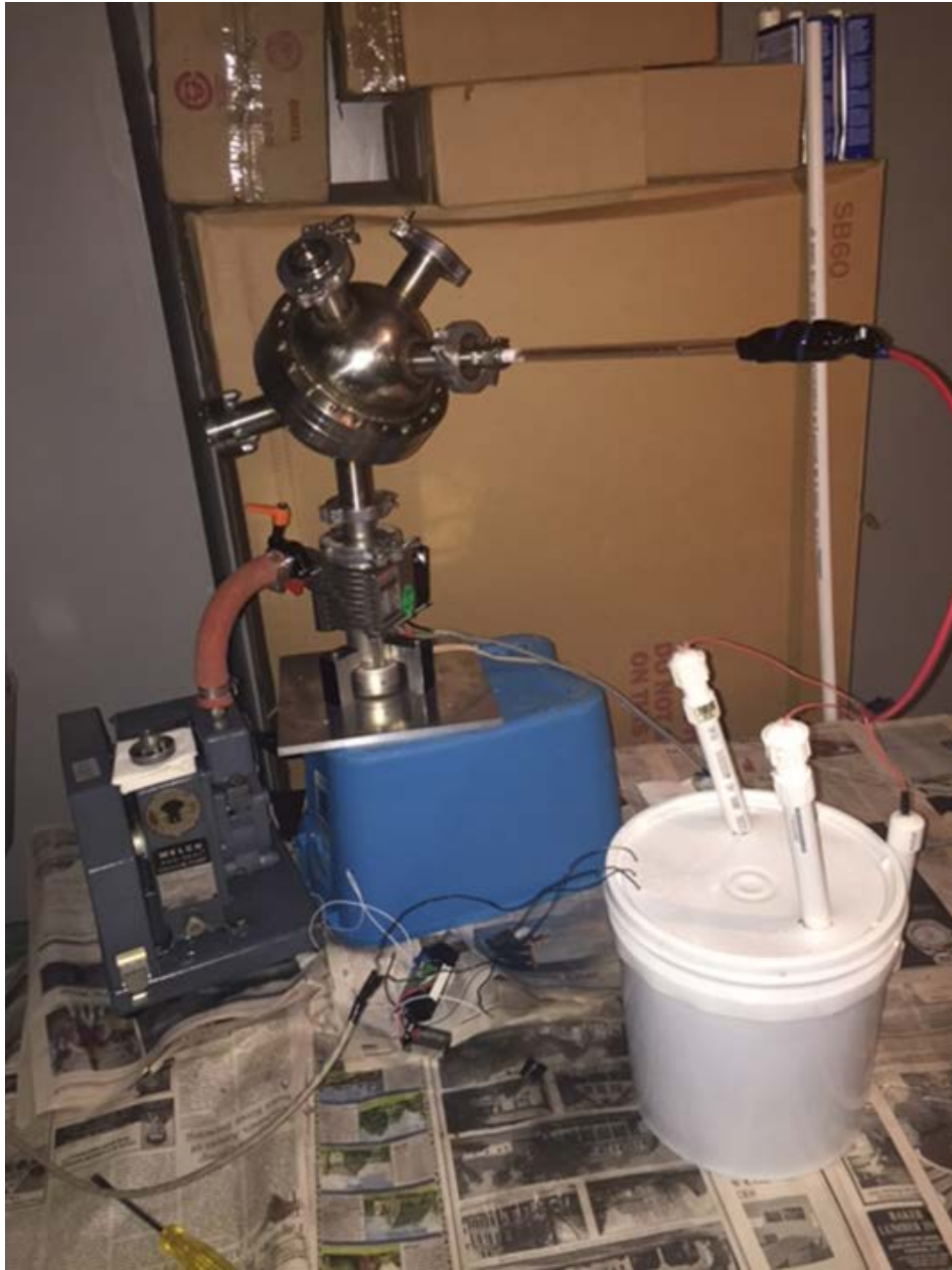
Chamber, High Voltage Supply, and Vacuum System
