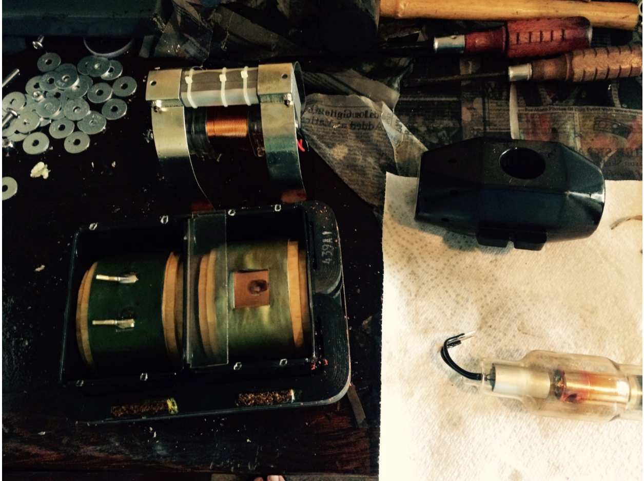
Disassembled X-Ray Head with High Voltage Transformer, Current Transformer, and Tube
