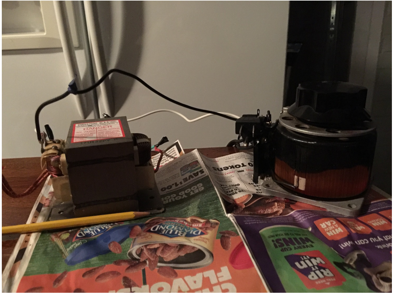
Autotransformer and Inductive Ballast
